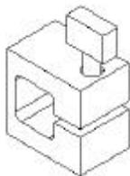
The second accessory to help with placement of the PALM Probe is a Locator Kit. The Locator Kit is mounted on the
