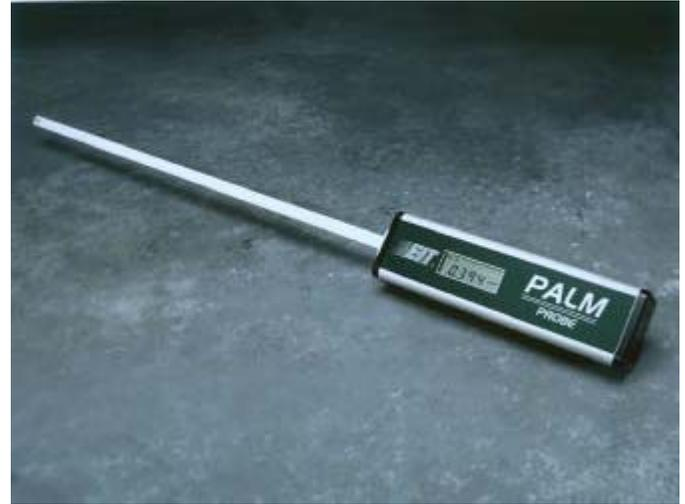
Light Guide to the base of the Probe body where the UV filter passes the UV light of interest to the photodetector. The photodetector converts the light energy to a current that is proportional to its intensity. The signal is conditioned, digitized, processed and displayed on the LCD of the PALM Probe.
